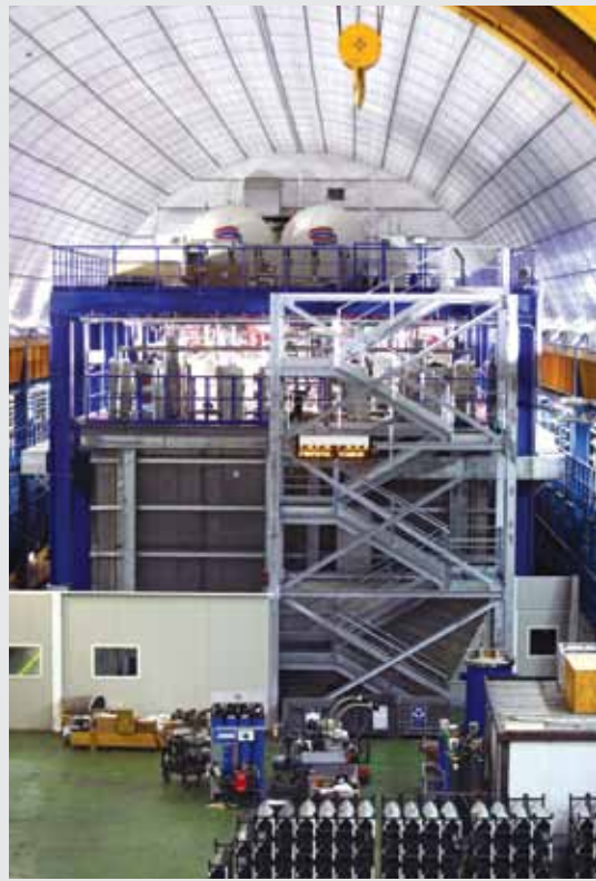
The ICARUS experiment at Italy's Gran Sasso National Laboratory is a pioneer in the use of liquid-argon technology to detect neutrinos. Like a bubble chamber from the early days of particle physics, the 600-ton detector allows scientists to record the tracks of the charged particles that a neutrino produces—but with electronics, rather than with photographs. Photo: Gran Sasso National Laboratory/INFN
