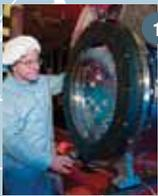
**1** Camera imager to measure galaxy distributions, supernovae, and distortions caused by dark matter. Designed and assembled at Fermilab.
