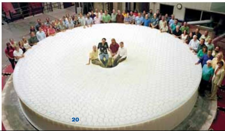
Members of the LSST corporation in 2008 with the completed cast, or blank, used to form the telescope's 27.5-foot-diameter primary mirror. The cast itself weighs 51,900 pounds.
