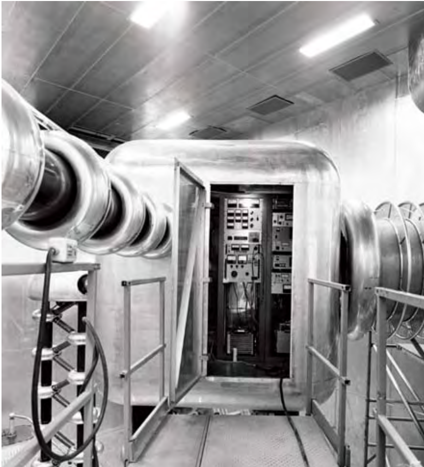
(above) Technicians Ray Hren and Jim Wendt helped build Fermilab's Cockcroft-Walton, and they serve as the main brains behind the machine's maintenance today. Hren (top photo, right) and Wendt were in their early 20s when they joined the laboratory in 1968. They were among the first technicians to be hired. (left) An open door reveals the inside of the equipment dome of the Cockcroft-Walton at Fermilab.
