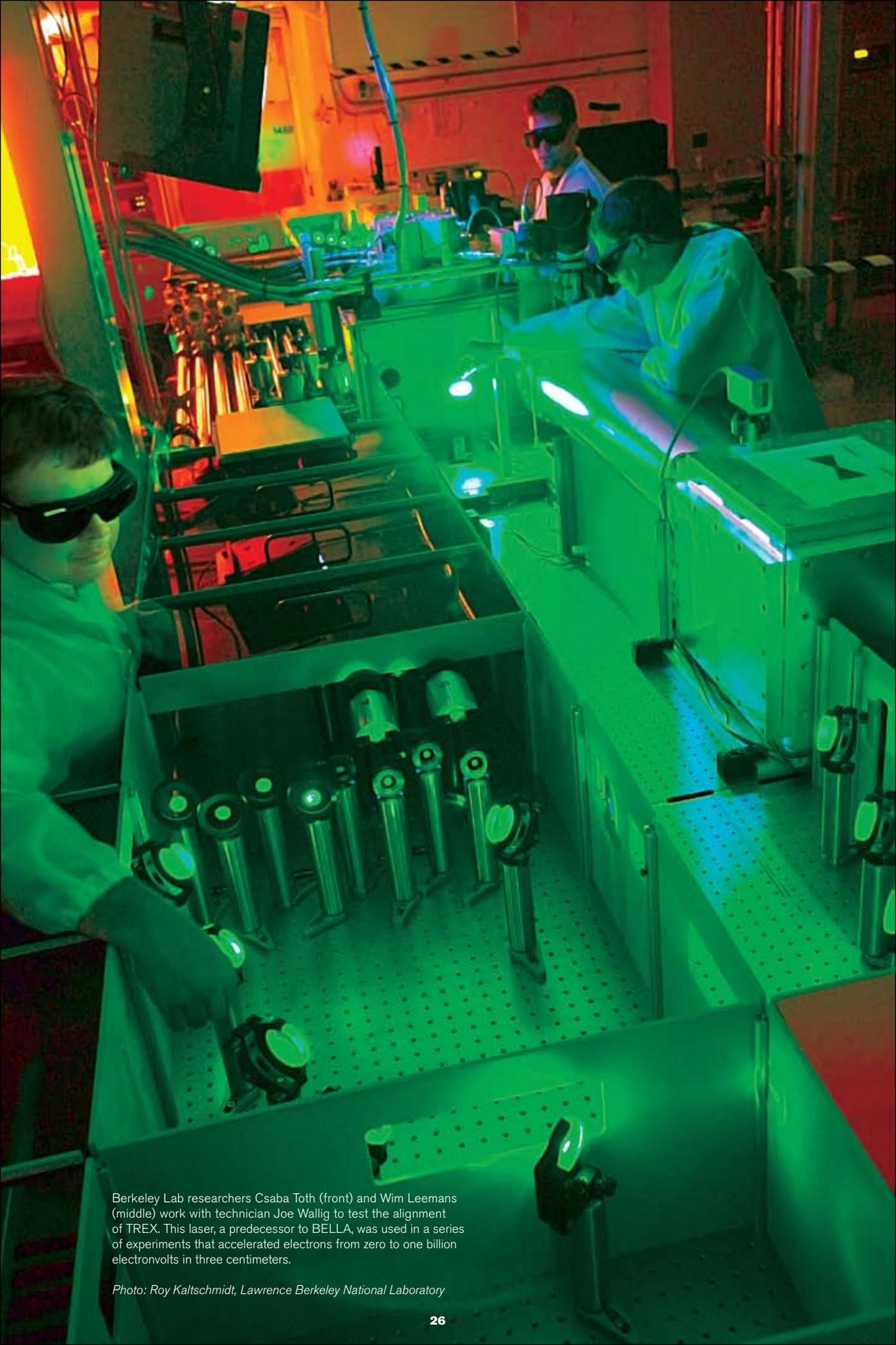
Berkeley Lab researchers Csaba Toth (front) and Wim Leemans (middle) work with technician Joe Wallig to test the alignment of TREX. This laser, a predecessor to BELLA, was used in a series of experiments that accelerated electrons from zero to one billion electronvolts in three centimeters.
