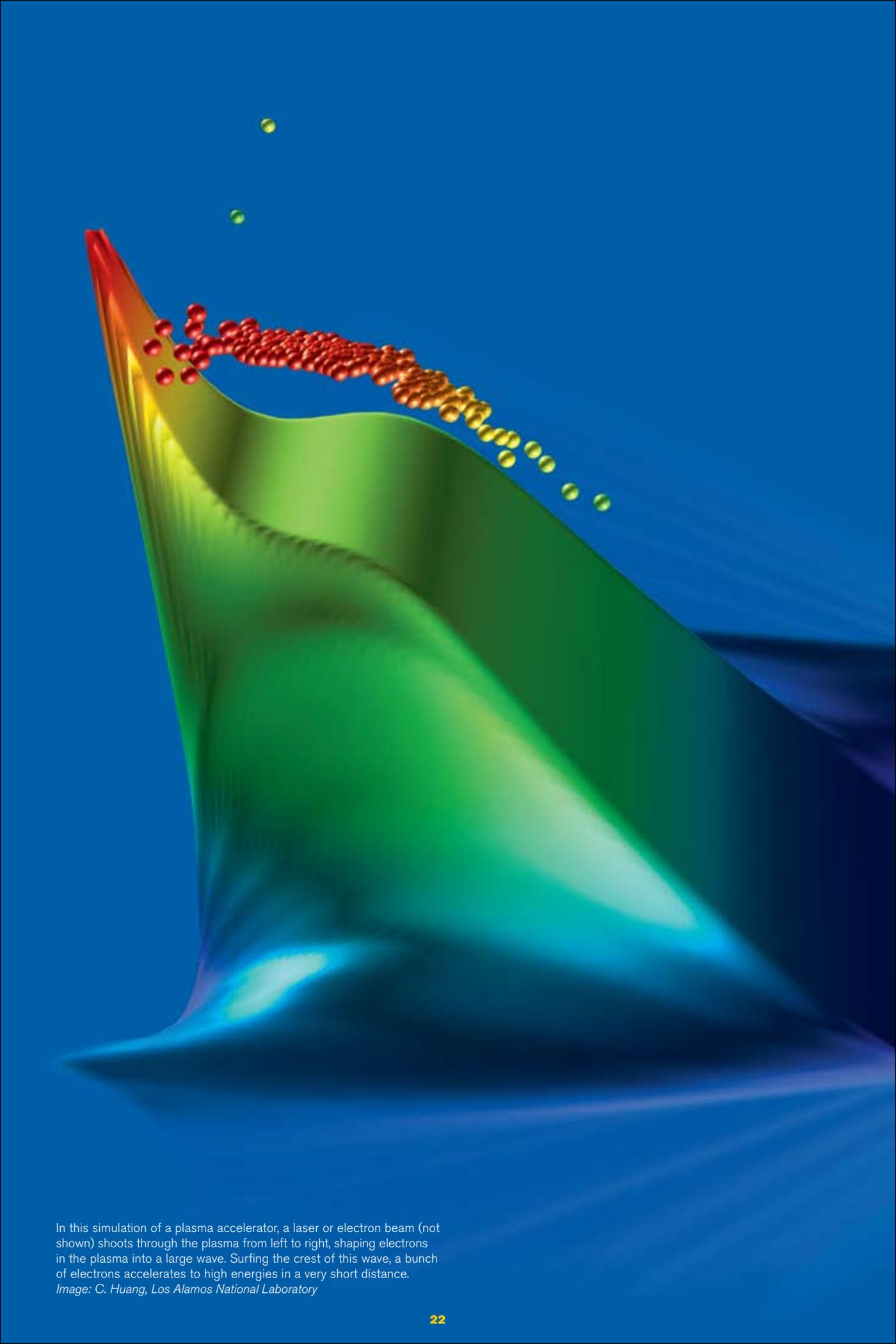
In this simulation of a plasma accelerator, a laser or electron beam (not shown) shoots through the plasma from left to right, shaping electrons in the plasma into a large wave. Surfing the crest of this wave, a bunch of electrons accelerates to high energies in a very short distance.
