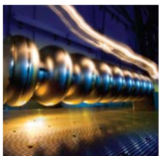
Left to right: superconducting cavities made of niobium; germanium crystal of the CDMS experiment; ATLAS silicon detector.
