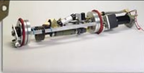
An improvised grinder sanded welds along the long, straight sections of 10,000 feet of pipe at Fermilab. The sander within the rotating silver cylinder cleaned each weld.
