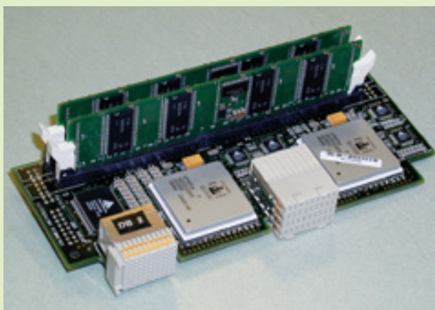
A QCDOC daughter card with two processing nodes and two 128 MB memory modules.
