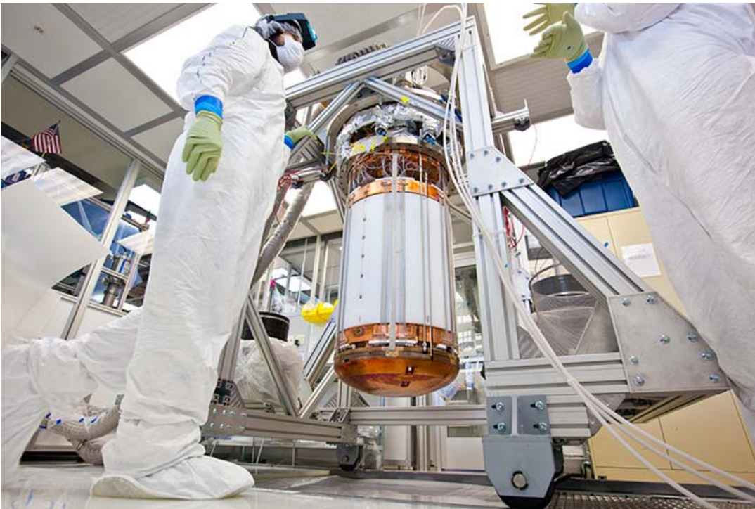
The LUX dark-matter detector, which scientists assembled and tested in a clean room above ground, is one of two physics experiments that will be installed 4850 feet underground in the new science facility this summer. Photo: Matt Kapust
