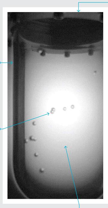
The biggest limitation for bubble chambers of the past was an inability to keep the **liquid** in a superheated state for an extended period of time. This required operators to time short blasts of particles from an accelerator to the few milliseconds when the temperature was just right. The COUPP collaborators got around this by finding a way to keep their liquid on the verge of boiling 80 percent of the experiment time, increasing the probability of catching dark matter particles.
