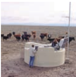
Workers at one of the observatory's 1500 surface detectors draw the attention of a herd of cattle. Each detector contains 3000 gallons of water; when particles from a cosmic ray shower pass through the water, their shock waves produce Cherenkov light that is measured by photomultiplier tubes. The resulting signal is automatically transmitted via radio. Solar panels generate 20 watts of power needed to run the detector.
