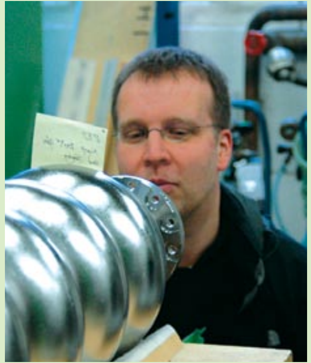
The International Linear Collider will use 16,000 superconducting cavities to accelerate electrons and positrons to 99.9999999998 percent of the speed of light.
