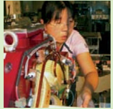
Magnets will keep particles on course as they zoom through the machine.
