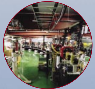
KEK's Advanced Test Facility is the forefront of low-emittance and high intensity beam steering technology. These technologies are essential for the proposed ILC. Seen in the photo is the northwest part of the ATF damping ring, with the arc section of the ring and the beam extraction line in the background.
