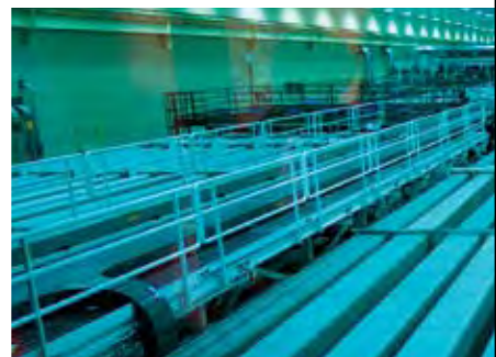
(Above) One of two laser bays at Livermore's National Ignition Facility, where 192 powerful lasers are focused onto a target the size of a pin in an attempt to cause nuclear fusion. (Far right) Nick and Lizzie at Fermilab; photo by Kurt Riesselmann. (Lower right) Los Alamos's proton radiography imager uses protons instead of photons to make detailed internal images of small explosions, allowing scientists to test aging nuclear weapons without detonating them.
